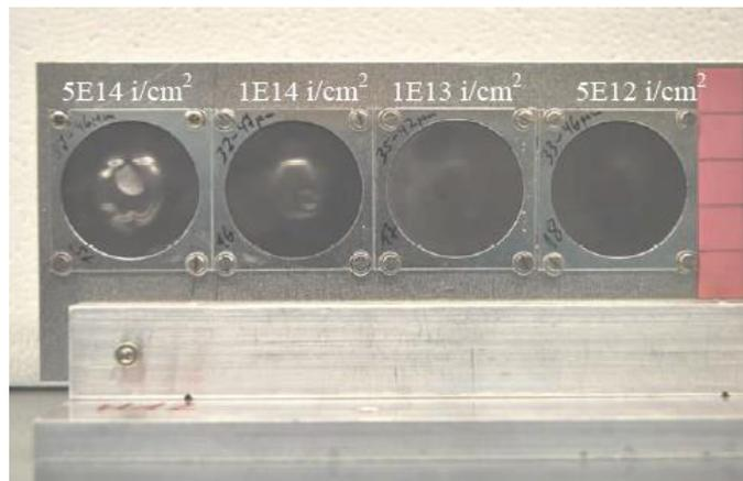
Fig. 1 – Failure of graphite target foils exposed to  $5 \times 10^{14} \text{ }^{238}\text{U}$  ions/ $\text{cm}^2$ , 150  $\mu\text{s}$  pulse length, 0.4 Hz, 4.8 MeV/u
