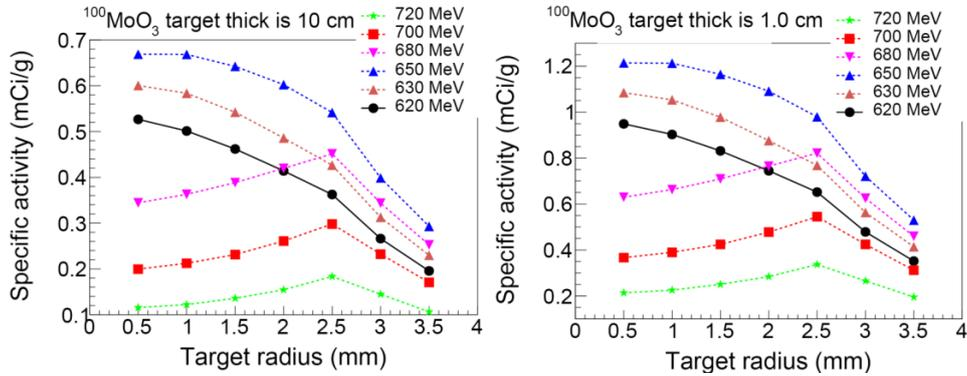
Fig. 11 – Saturation specific activity as function of the target radius while its thickness is 10 cm (left) and 1.0 cm (right), respectively.
