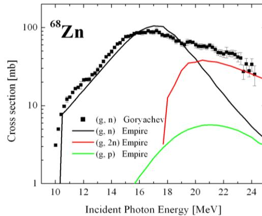
Fig. 14 – Simulation of nuclear reaction  $^{68}\text{Zn}(\gamma, n)$  and of competing reactions.
