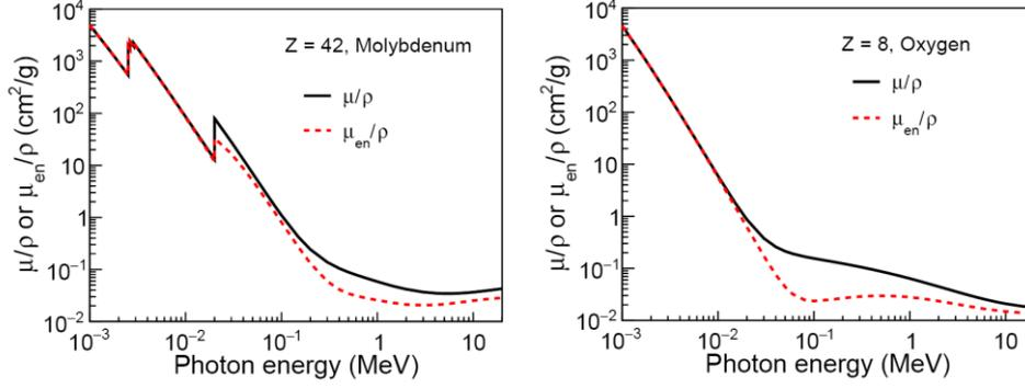
Fig. 6 – The attenuation coefficients of  $^{100}\text{Mo}$  and  $^{16}\text{O}$  [24]. Since a thick target (molybdenum oxide, *i.e.*  $\text{MoO}_3$ ) would be employed to produce radioisotopes, the attenuation coefficient should be fully considered in the simulation.
