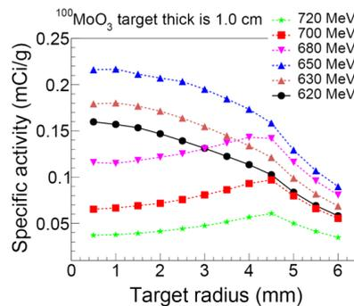
Fig. 12 – Specific activity as a function of target radius for a 16.4 m distance between the IP and the isotope target.
