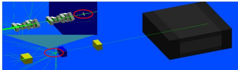
Fig. 3 – The set-up of  $\gamma$ -ray beam transport in Geant4. The inserted figure in the top left corner represents the enlarged collimator and target zone.
