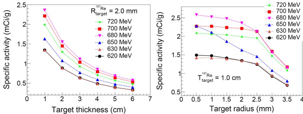
Fig. 22 – Saturation specific activity of the  $^{186}\text{Re}$  radioisotope as function of the target thickness (left) and radius (right) for different e-beam energies.
