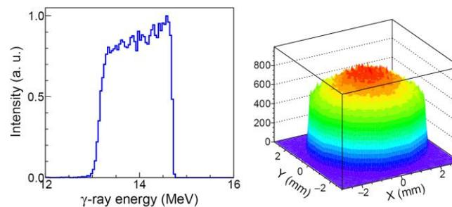
Fig. 4 – A  $\gamma$ -ray beam spectrum (left) and transverse profiles (right) on the surface of the target.
