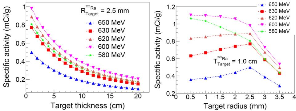
Fig. 18 – Saturation specific activity of the  $^{225}\text{Ra}/^{225}\text{Ac}$  radioisotopes as function of the target thickness (left) and radius (right) for different  $e$ -beam energies.
