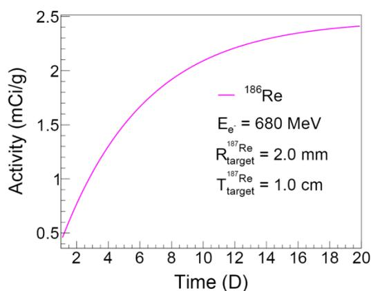
Fig. 21 – The specific activity of  $^{186}\text{Re}$  as a function of irradiating time. The target is choose to be 2.0 mm radius and 1.0 cm thick.
