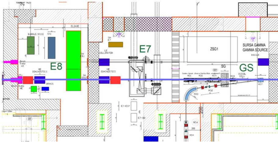
Fig. 23 – Position of the irradiation station for medical isotopes (red rectangular box) at the high-energy  $\gamma$ -beam line (in blue) in E7 and E8 experimental areas.
