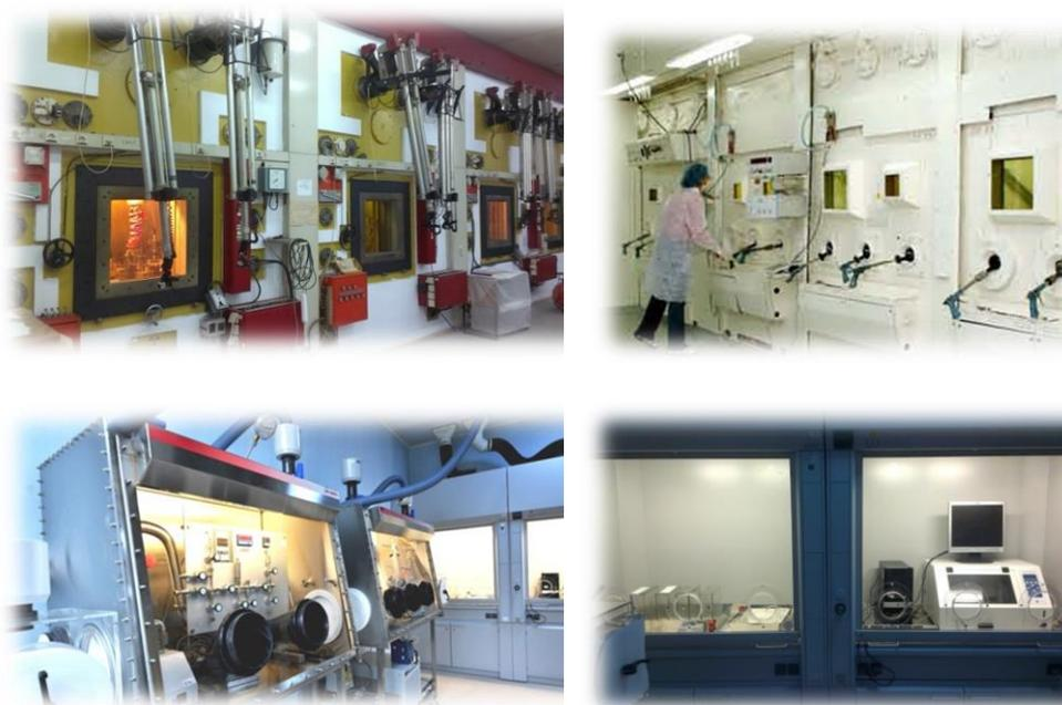
Fig. 24 – Some of the hot cells and radiochemistry hoods installed at IFIN-HH.
