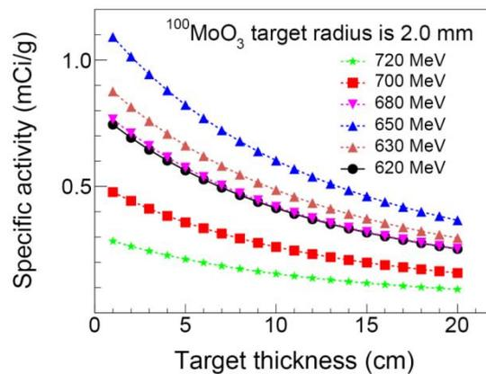
Fig. 10 – Saturation specific activity as function of the target thickness.
