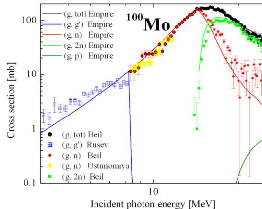
Fig. 5 – Simulation of nuclear reaction  $^{100}\text{Mo}(\gamma, n)$  reaction and of competing reactions. The experimental cross section is also shown for comparison. The maximum  $(\gamma, n)$  reaction cross section is 150 mb corresponding to the incident  $\gamma$ -ray energy,  $E_\gamma=14.5$  MeV.
