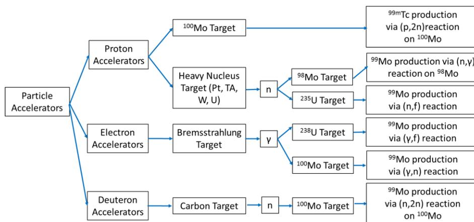
Fig. 7 – Alternative methods of producing Mo-99 using accelerators.
