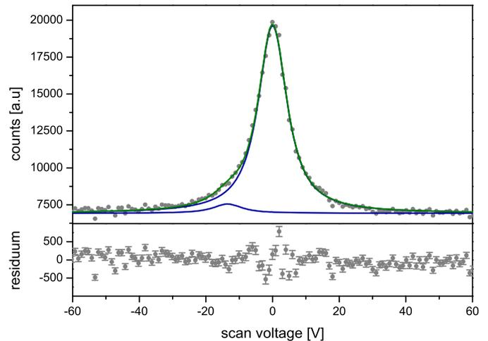
**Fig. 1.** Spectrum of the reference isotope  $^{114}\text{Cd}$  in the  $5s\ 5p\ ^3P_2 \rightarrow 5s\ 6s\ ^3S_1$  transition. The fitted curve is the sum of two Voigt profiles – also shown individually – with a relative position of 13.5 V to each other. The lower panel shows the residuum between the experimental data and the fit. Typical total linewidth (Lorentzian + Gaussian contribution) is about 30–40 MHz.
