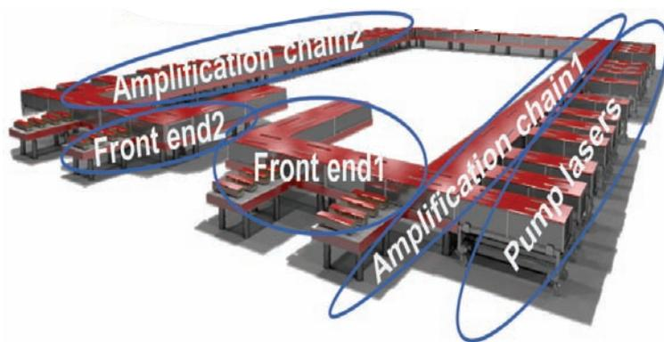
**Figure 3.** Schematic layout of the ELI-NP High Power Laser System (HPLS).
