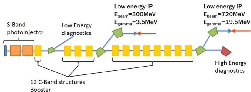
**Figure 4.** General layout of the ELI-NP Gamma Beam System (GBS).
