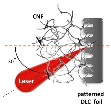
**Figure 2.** Spaghetti-like carbon nanotubes grown on patterned DLC.
