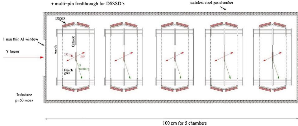
**Figure 2.** Schematic representation of a five-fold Frisch-gridded twin ionization chamber.
