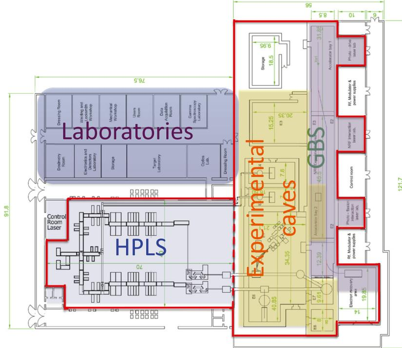
**Figure 1.** Lay-out of the ELI-NP laboratory building. The dimensions are in metres. The bold contour indicates the borders of the antivibration slab.
