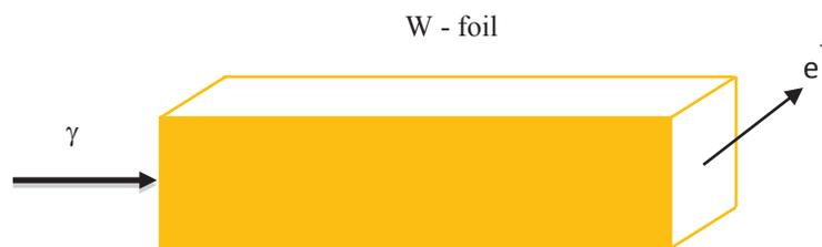
**FIGURE 1.** Sketch of a simple W converter foil irradiated with a  $\gamma$  beam for positron–electron pair production.
