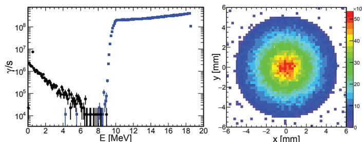
**FIGURE 1.** Left: spectrum of the  $\gamma$  beam (blue squares) collimated below 0.7 mrad and background photon spectrum (black circles) generated in collimator. Right: the collimated gamma beam spot at 775 cm, with a standard deviation  $\sigma(1D)=2.1$  mm.
