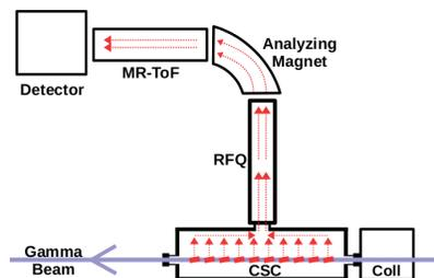
**FIGURE 2.** Conceptual drawing of the layout of the IGISOL beam line: target foils are shown with full red lines and ion trajectories are shown with dashed red arrows.
