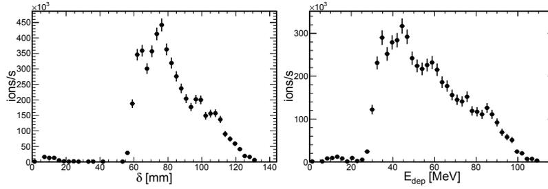
**FIGURE 4.** Left: total path length  $\delta$  of the ions released from the target in the gas cell. Right: energy deposited  $E_{dep}$  by the ions released from the target in the gas cell.
