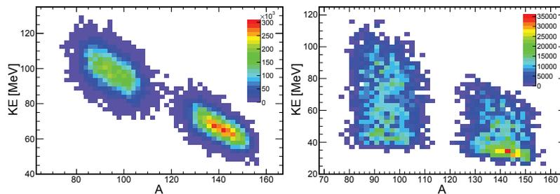
**FIGURE 3.** Left: kinetic energy KE versus atomic mass A of photofission fragments produced in the target. Right: kinetic energy KE versus atomic mass A of photofission fragments released from a target with  $7\ \mu\text{m}$  thickness. Both correspond to a total rate of  $1.7 \cdot 10^7$  fissions/s produced by exposing 800 mg of  $^{238}\text{U}$  to  $5 \cdot 10^{10}\ \gamma/\text{s}$ .
