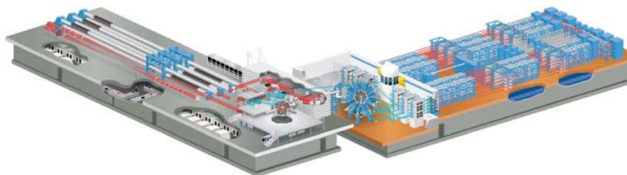
Fig. 1. The OMEGA EP and OMEGA 60 Laser Systems are shown on the left and right, respectively. Each system contains a target chamber for experiments and selected beams from OMEGA EP can be directed to the OMEGA 60 chamber for joint operations
