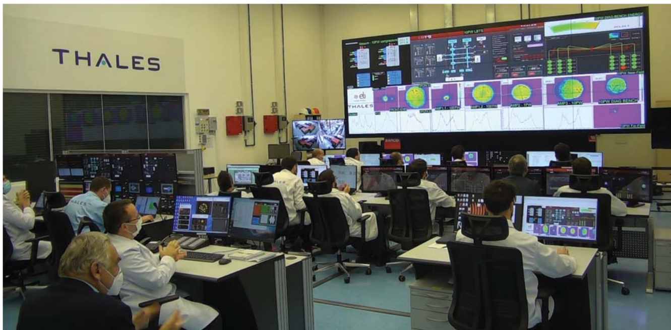
The laser shot demonstration at 10 PW output. The large display screen showed various laser data such as the near and far field patterns, spectrum bandwidth, and output laser energy
