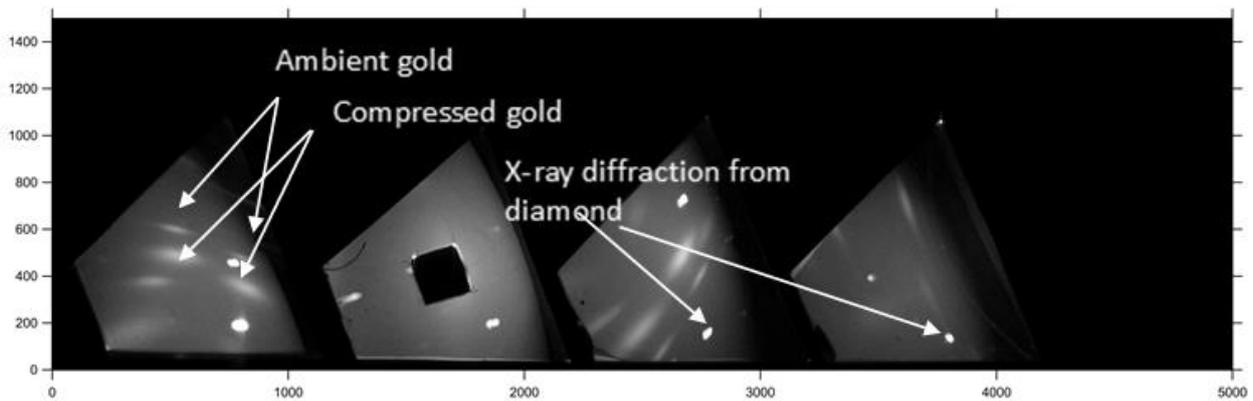
Figure 2: X-ray diffraction data from strongly textured gold.
