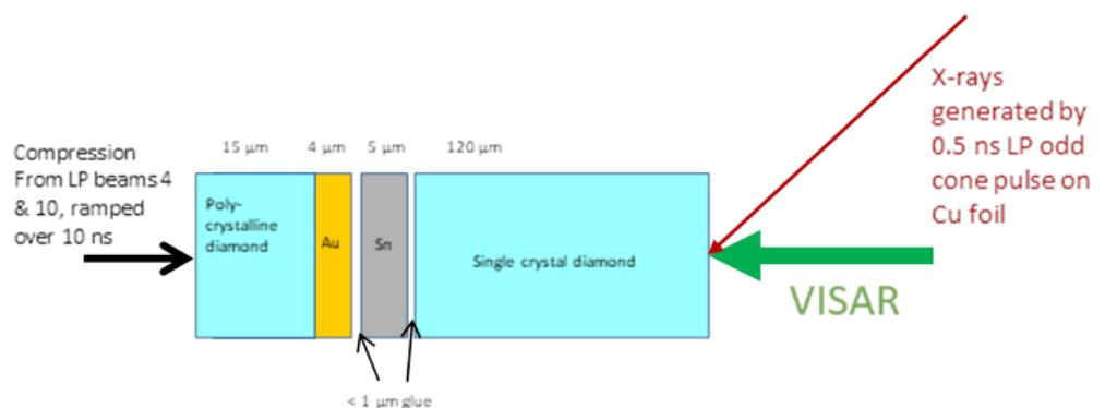
Figure 1: Experimental platform showing how materials are compressed to high pressures in diamond sandwiches.
